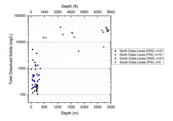
Figure 4.16. Total dissolved solids concentrations of aqueous samples from water wells (WW) (solid circles) and production wells (PW) (hollow circles) in oil fields in the West Kern Valley Floor subregion as a function of the lower perforation and upper perforation depths of water and production wells, respectively. Source: Data from Metzger et al. (2018).
