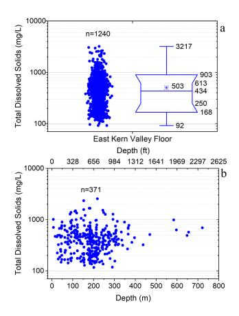
Figure 4.9. Concentrations of TDS in water wells with 3.2 km of oil production wells in the East Kern Valley Floor subregion. (a) Box plot illustrating distribution of values: the asterisk denotes the mean concentration. Values outside the box plot in ascending value denote minimum, 10%, 25%, 50% (median), 75%, 90%, and maximum values. (b) Total dissolved solids concentration as a function of the lower perforation depth of water wells. Source: Metzger et al. (2018).
