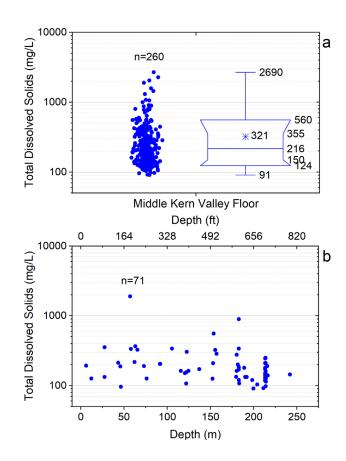
Figure 4.11. Concentrations of total dissolved solids in water wells within 3.2 km of oil production wells in the Middle Kern Valley Floor subregion. (a) Box plot illustrating distribution of values: the asterisk denotes the mean concentration. Values outside the box plot in ascending value denote minimum, 10%, 25%, 50% (median), 75%, 90%, and maximum values. (b) Total dissolved solids concentration as a function of the lower perforation depth of water wells. Source: Metzger et al. (2018).
