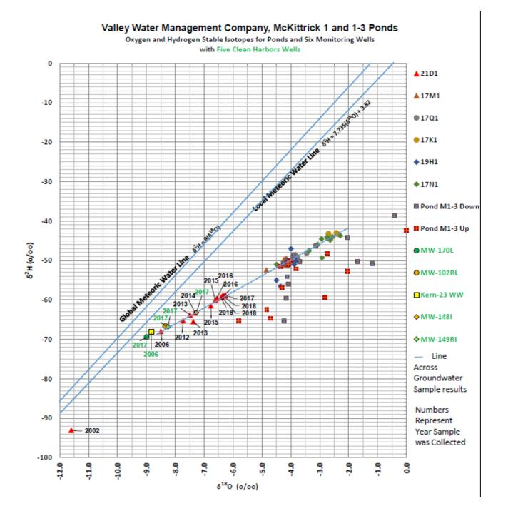
*Figure 4.23. Water isotope figure of produced wastewater and groundwater wells. Source: CVRWQCB (2019).*
