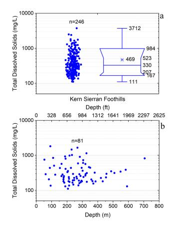
Figure 4.7. Concentrations of total dissolved solids in water wells within 3.2 km of oil production wells in the Kern Sierran Foothills subregion. (a) Box plot illustrating distribution of values: the asterisk denotes the mean concentration. Values outside the box plot in ascending value denote minimum, 10%, 25%, 50% (median), 75%, 90%, and maximum values. (b) Total dissolved solids concentration as a function of the lower perforation depth of water wells. Source: Metzger et al. (2018).
