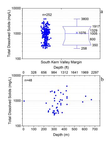
Figure 4.13. Concentrations of total dissolved solids in water wells within 3.2 km of oil production wells in the South Kern Valley Margin subregion. (a) Box plot illustrating distribution of values: the asterisk denotes the mean concentration. Values outside the box plot in ascending value denote minimum, 10%, 25%, 50% (median), 75%, 90%, and maximum values. (b) Total dissolved solids concentration as a function of the lower perforation depth of water wells. Source: Metzger et al. (2018).
