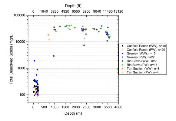
Figure 4.12. Total dissolved solids concentrations of aqueous samples from water wells (WW) (solid circles) and production wells (PW) (hollow circles) in oil fields in the Middle Kern Valley Floor subregion as a function of the lower perforation and upper perforation depths of water and production wells, respectively. Source: Metzger et al. (2018).
