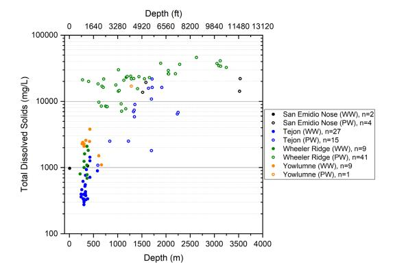
Figure 4.14. Total dissolved solids concentrations of aqueous samples from water wells (WW) (solid circles) and production wells (PW) (hollow circles) in oil fields in the South Kern Valley Margin subregion as a function of the lower perforation and upper perforation depths of water and production wells, respectively. Source: Data from Metzger et al. (2018).
