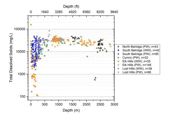
Figure 4.18. Total dissolved solids concentrations of aqueous samples from water wells (WW) (solid circles) and production wells (PW) (hollow circles) in oil fields in the West Kern Valley Margin subregion as a function of the lower perforation and upper perforation depths of water and production wells, respectively. Source: Data from Metzger et al. (2018).
