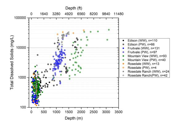
Figure 4.10. Total dissolved solids concentrations of aqueous samples from water wells (WW) (solid circles) and production wells (PW) (hollow circles) in oil fields in the East Kern Valley Floor subregion as a function of the lower perforation and upper perforation depths of water and production wells, respectively. Source: Metzger et al. (2018).
