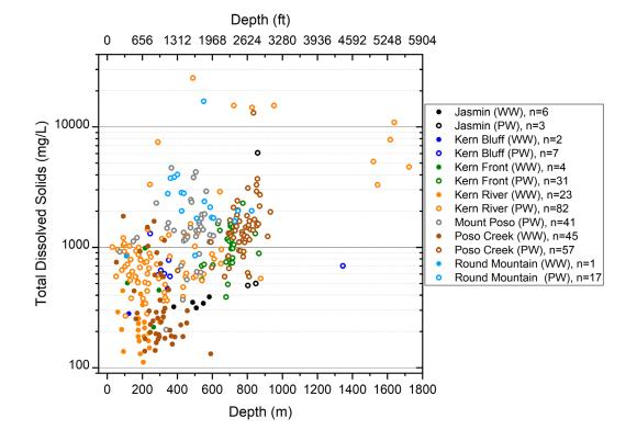
Figure 4.8. Total dissolved solids concentrations of aqueous samples from water wells (WW) (solid circles) and production wells (PW) (hollow circles) in oil fields in the Kern Sierran Foothills as a function of the lower perforation and upper perforation depths of water and production wells, respectively. Source: Data from Metzger et al. (2018).
