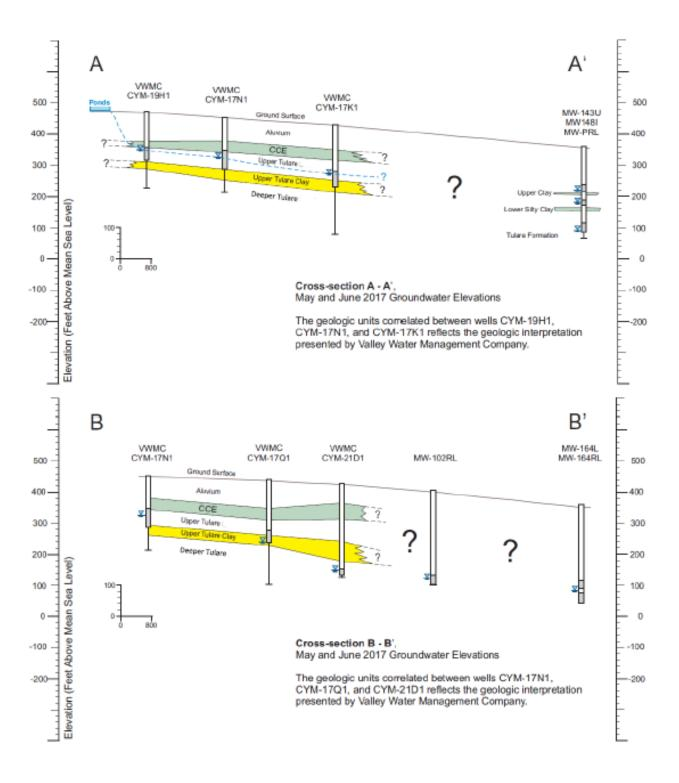
Figure 4.21. Cross-sectional schematic A–A' from Figure 4.20 illustrating stratigraphy and the possible extent of migration of produced water in the Upper Tulare Sand above the Upper Tulare Clay. Source: CVRWQCB (2019).
